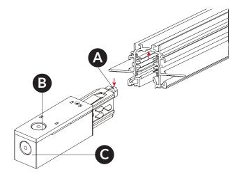
In order to correctly wire the system, the End Feed has a mechanical key / groove (A) that ensures the correct insertion into the track. When installing, ensure that the mechanical key is oriented properly.
